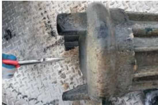
Pumps have a hard time with wipes and other large solid materials. As seen above this pump is plugged and required maintenance actions. Pumps are not the only thing to plug. Residential sewer lines are typically small four-inch lines and can be plugged; causing costly backups into your home. These issues can be avoided by throwing away and not flushing these following items:
